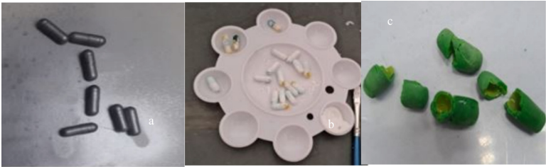
Fig. 4. Coatings of capsules through different materials (a) Spray-painted capsules (b) Acrylic-painted capsules (c) Breakage of play-dough coated capsules
