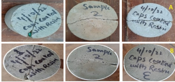
Fig. 8. Split samples with respect to days of healing (a) 0 day (b) 14 day
