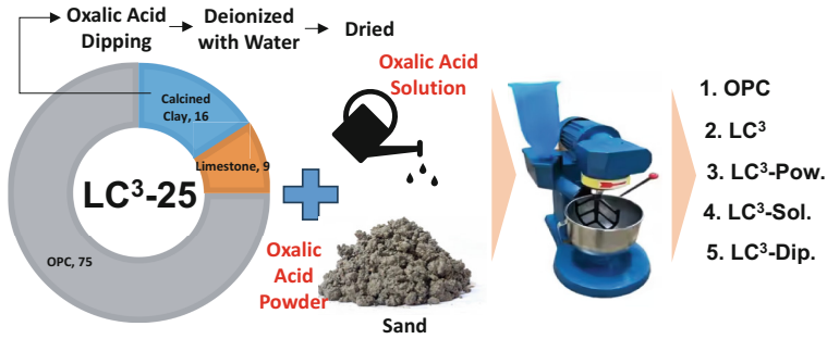
Fig. 1. Type of specimen prepared in this work.
