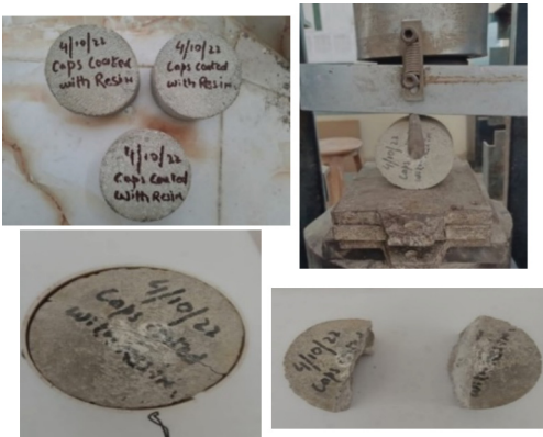
Fig. 7. Step-by-step procedure for pre-cracking
