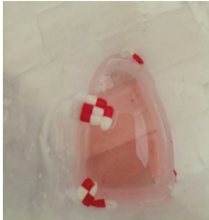
Fig. 3. Distortion of capsules immersed in water
